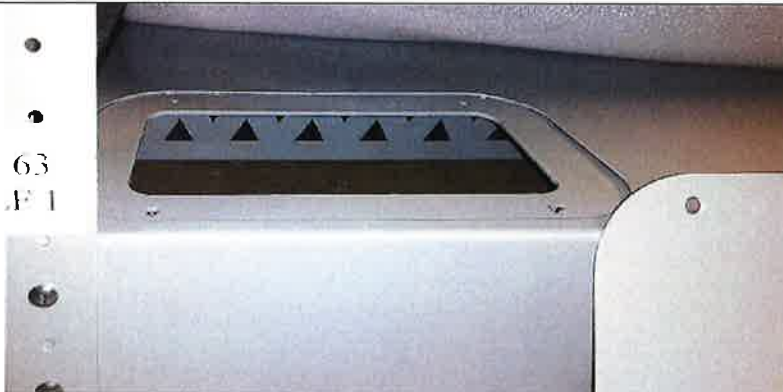
Image #13 – 4" high x 36" wide support brace running underneath the bottom base shelf
