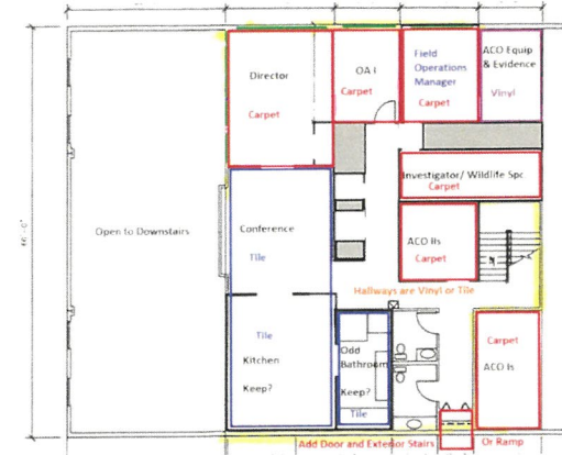
Second Floor Renovated Plan Includes Flooring(NTS)
